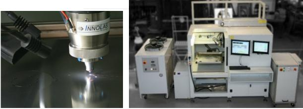
We custom design each of our Class 1 laser work enclosures to suit the particular installation. Direct or fibre optic beam delivery and advanced through-the-lens camera systems ensure the laser beam is always on target. All laser parameters are controlled via our simple-to-use PC software, touch-screen or hand-held controllers. Multi-axis motion control, shield- or assist-gas delivery, fume extraction, vision systems and interlocked access are all individually specified.
